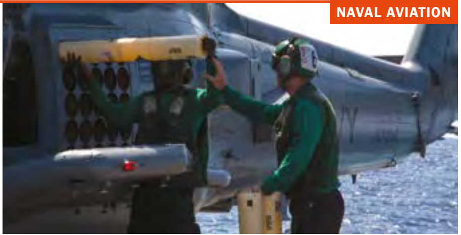
US Navy technicians unload sonobuoys from an MH-60R Sea Hawk on the flight deck of the guided-missile destroyer, USS Mason (DDG 87). (Photo: US Navy)
