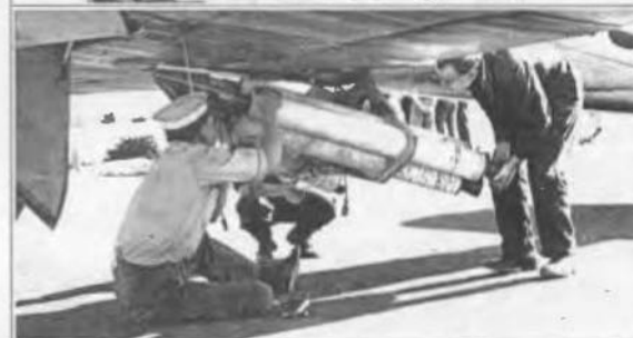
JERVIS BAY AIRFIELD 1950 Armourers assembling and fitting RATOG equipment All photographs this page courtesy AMoF
