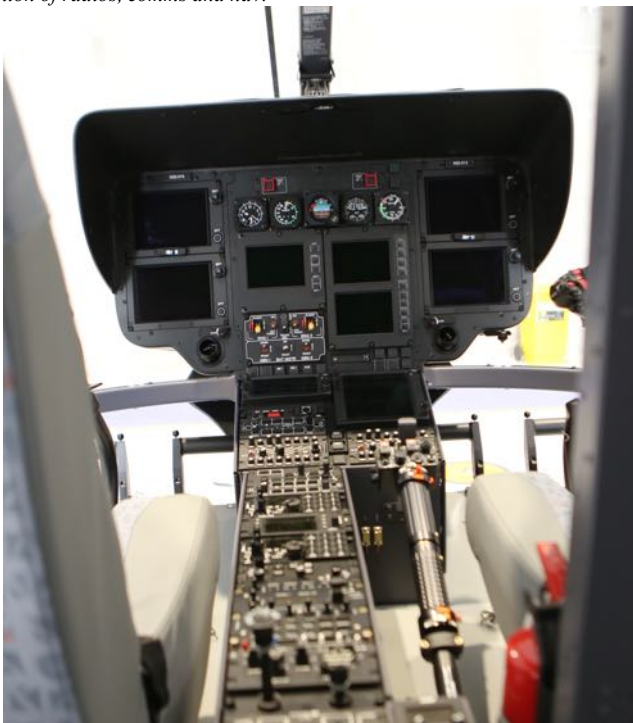
Below: The EC135 cockpit. Pilot flying displays are the large screens top LH and RH side. Below them are the Navigation Displays. The three screens in the centre front panel are the Caution Advisory Display on the left and the two Vehicle Engine Management Displays, one above the other (shows Ts&Ps, for you old aviators!). Between the seats console is the usual collection of radios, comms and nav.
