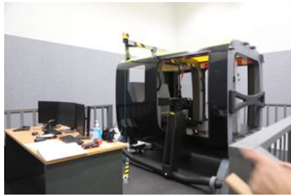
Left. An EC135T2 undergoing maintenance in the immaculate hangar. Centre. The Aircraft Replica Trainer, which uses Virtual Reality to teach winching. Right: the Marshalling Trainer, which also uses VR.
