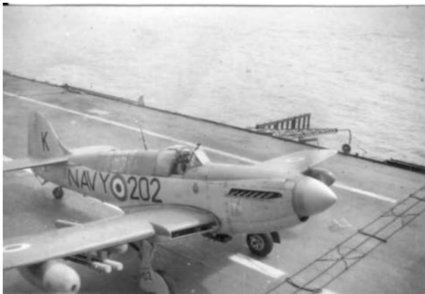
Fairey Firefly AS Mk 6, 817 Squadron RAN. Probably in February 1955 aboard the aircraft carrier HMAS Sydney. The aircraft is taxiing to the catapult prior to launch for rocket projectile firing. The aircraft is armed with four rocket projectiles with 60lb concrete heads. (Pilot and photo: John van Gelder)
