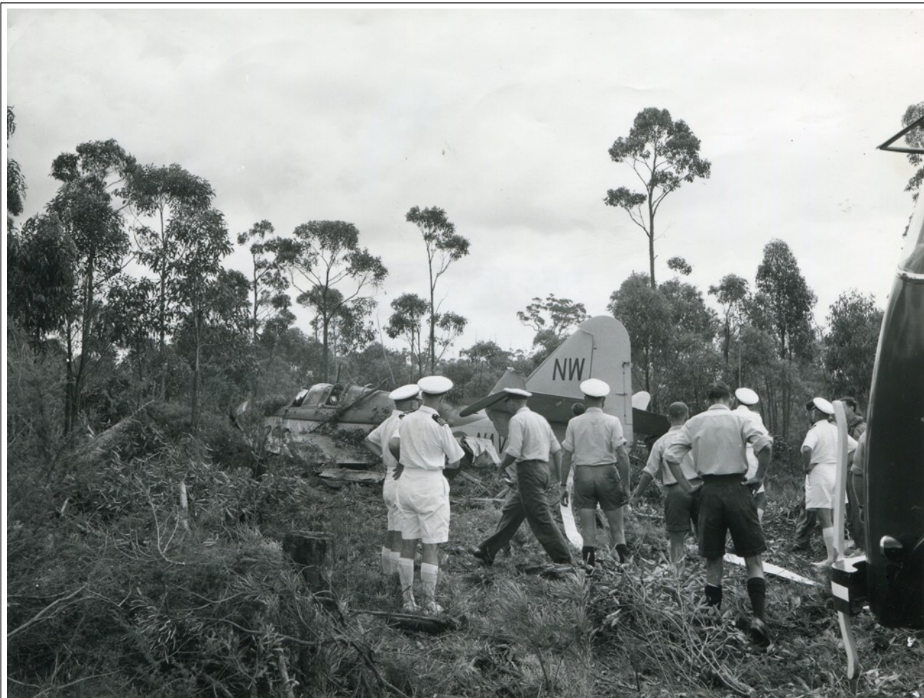
Gannet XA330 was lost in February of 1961 when the pilot allegedly lowered the undercarriage during a single engine landing, without selecting the Flight Fine Pitch Stop on for the live engine.
