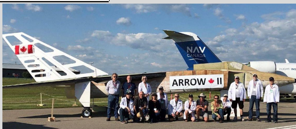
The 60% scale Avro Arrow II on the tarmac at Springbank Airport in Calgary, Canada. With a projected cost of $1.5m the build is about 70% complete. The aircraft is designed to fly at 500 knots with a 12,000 fpm Rate of Climb, with two people on board.
