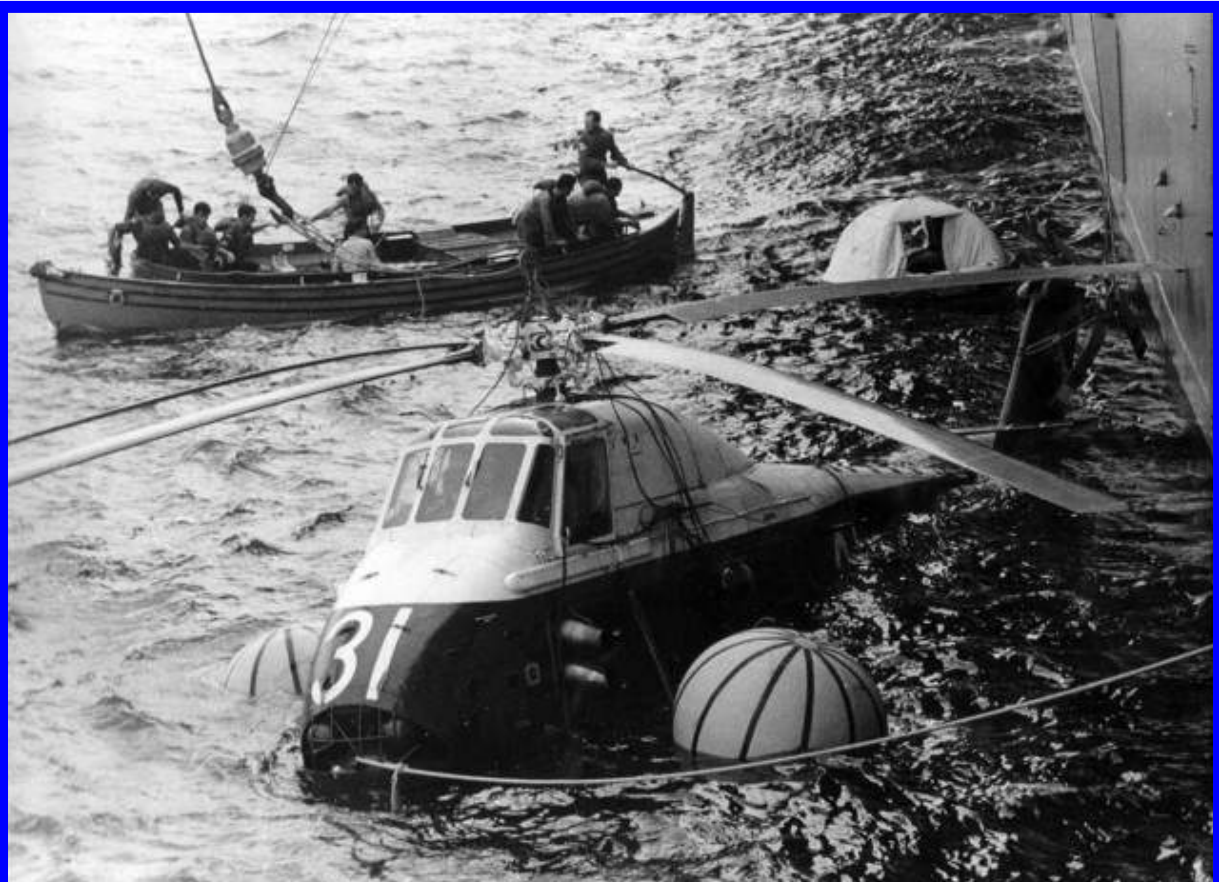
Wessex N7-221 in the drink after an engine failure from HMAS Melbourne
