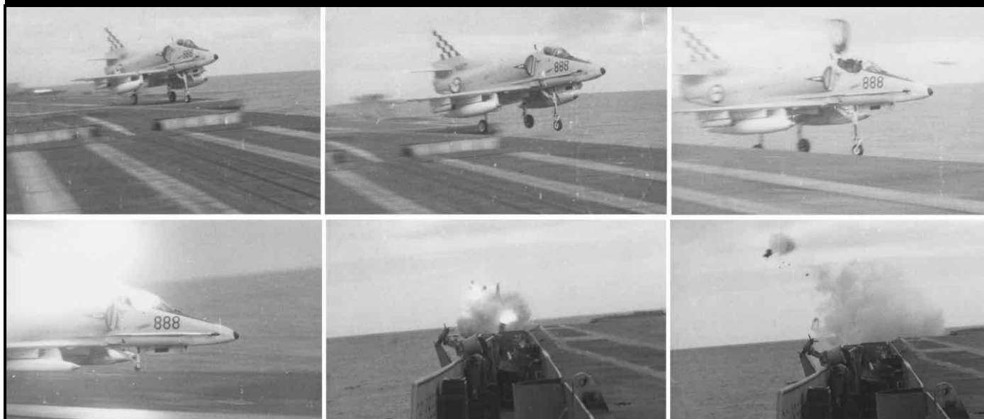
Lieutenant Commander Kevin Finan's USN spectacular ejection from Skyhawk 888 following an arrestor wire failure
