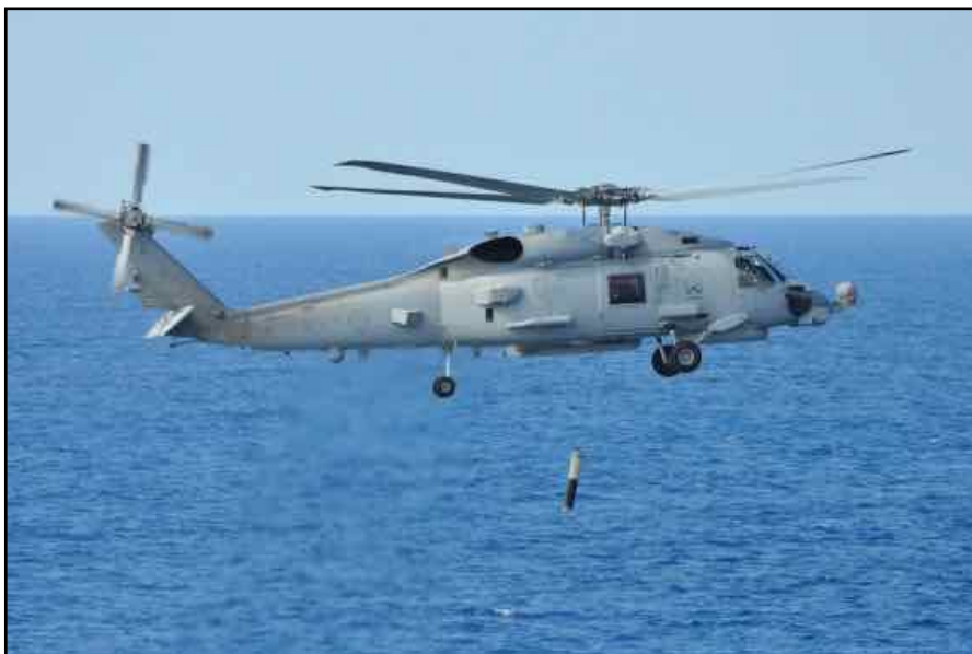
The RAN's MH-60R Romeo helicopter conducts functional testing of the newly fitted Airborne Low Frequency Sonar System (ALFS) off the coast of Jacksonville, Florida.
