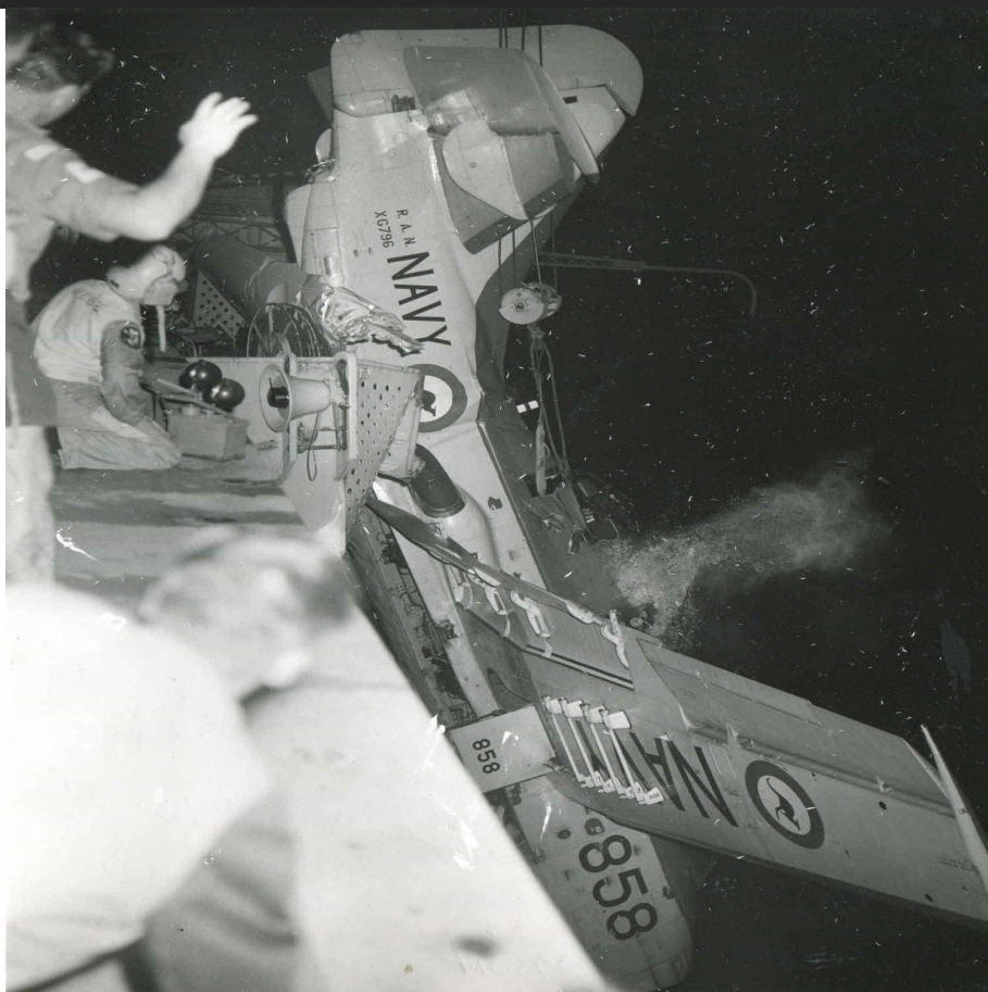
XG796 hanging over side of HMAS Melbourne with a strop attached to ship's crane. Unfortunately, this failed and aircraft fell into sea.
