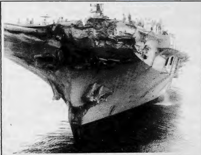
The extent of the above water damage to Melbourne's bows can be clearly seen. The heat generated by the impact welded parts of the destroyer to the carrier. Photos RAN
