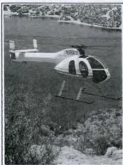
The McDonnell Douglas MD 520N is the first helicopter design to incorporate a radical concept known as NOTAR (No Tail Rotor). The tail rotor has been eliminated using the theory of the 'Coanda Effect', which basically states that air flowing over the curved tail boom of the helicopter follows the contour of its surface. The tailboom then acts like a wing, but instead of giving lift actually produces a sideways movement which is what the tail rotor is normally required for.
