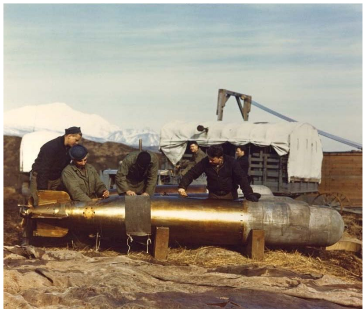
Above: A Mk 13 being serviced by USN ordnancemen, as they did at Nowra. The conditions were probably similar to this, which were hardly ideal for such a delicate machine. This appears to be an early model of the Mk13 as there is no propellor ring fitted. (Image: Public Domain).
