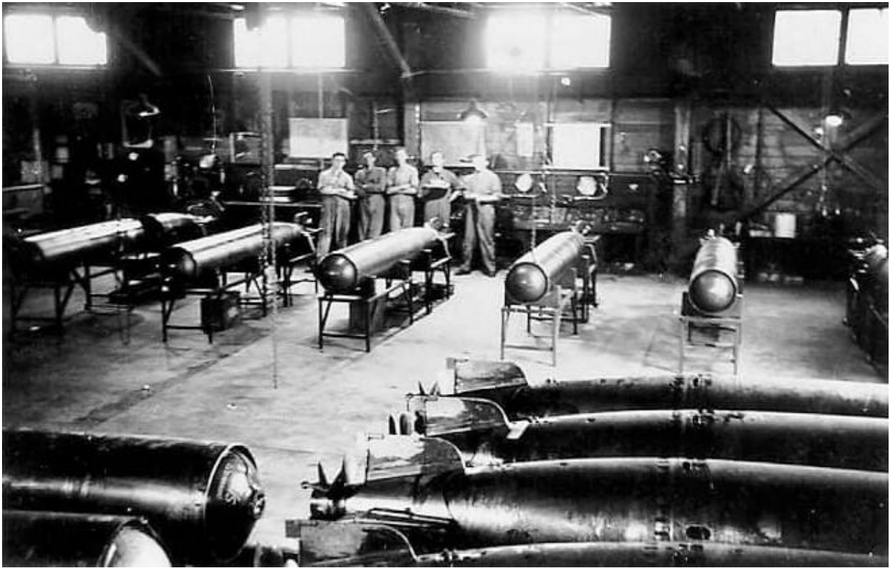
Above: A rare photo of the BTU workshop floor taken by SGT Alan Smith who was posted there from Oct43 to May 44. We are advised they are Mk.13 torpedoes but are missing the warhead assembly, which gives them a different look. The image gives a good idea of the rudimentary nature of the BTU facility. Image SGT Smith.
