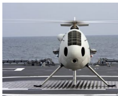
Far Left. The Boeing ScanEagle, designed for long endurance surveillance operations at sea. Left: the shorter range Schiebel S100 has a higher payload and VTOL capability off any small deck.
