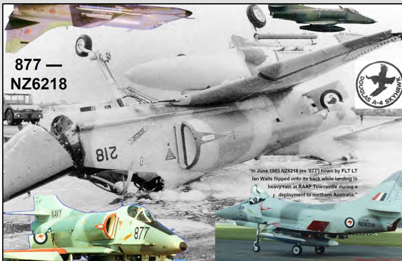
Below: 877, now rebadged as RNZAF NZ6218, flipped over whilst landing in a rainstorm at RAAF Townsville on 03 June 1985. The pilot was unhurt but the severely damaged aircraft required repatriation to New Zealand by C130 and almost five years of repair work, using the rear fuselage of an ex-USN 'Blue Angels' airframe. It was returned to (NZ) service on 23 March 1990, and subsequently sold to Draken International.
