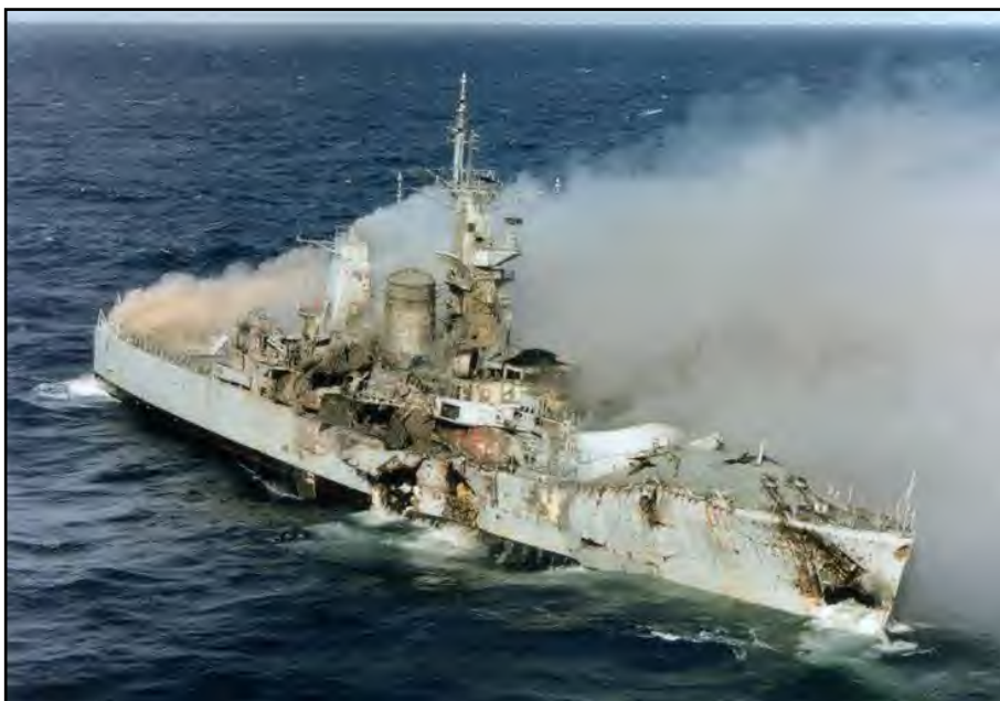
HMS Sheffield after an attack by two Super Étendard aircraft with one Exocet missile hitting the ship. Sheffield later sank.
