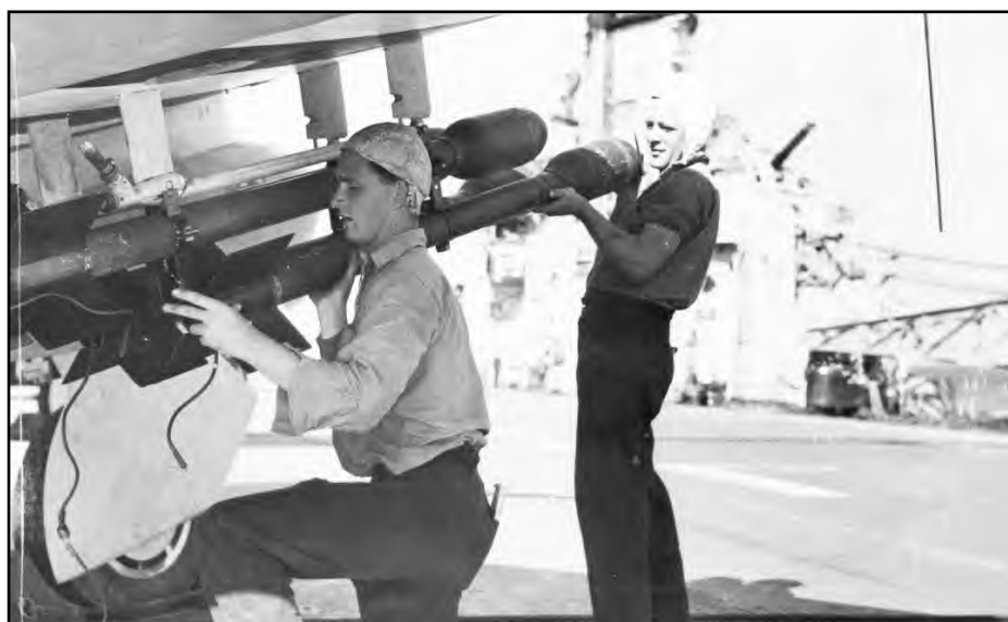
Naval armourers R. Lilly and K. Pascoe fix rockets to a Sea Fury prior to a mission
