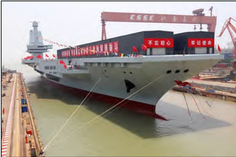
Chinese Aircraft Carrier (Type 003) named 'Fujian' launched on 17 June 2022. The ship is a conventional carrier around the size of the USS Kitty Hawk Class. Gross Tonnage estimated near 90,000 tons
