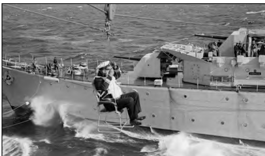
Rear Admiral Scott-Moncrieff transferring from HMAS Sydney to the C-class destroyer HMS Comus via a Jackstay transfer
