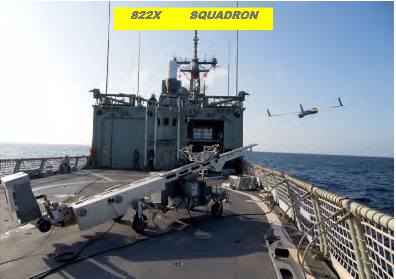
ScanEagle is launched from the flight deck of HMAS Newcastle in the Middle East region.
