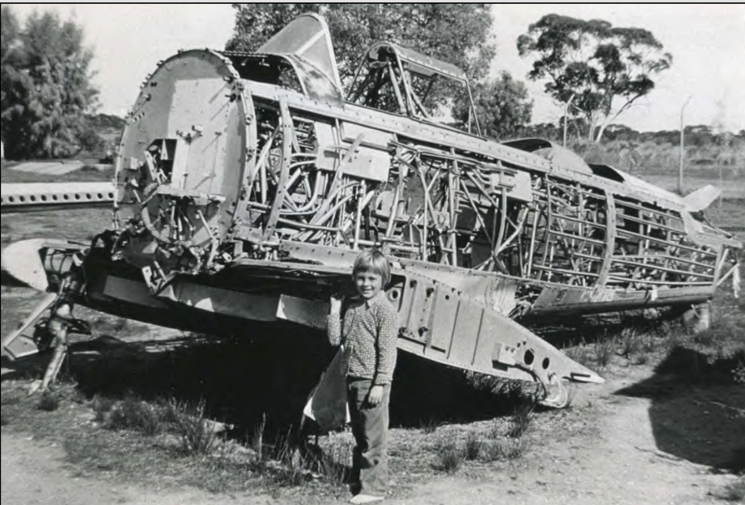
Above. Neither of these aircraft served in Navy, but their photos show useful features. On the left, this wreck near Mildura gives a good impression of the solidity of the Wirraway's construction. On the right: one of the few images we've seen with the gunner's position in the aft cockpit manned. (via FAAM). Below. A20-139 parked alongside a Sea Fury at NAS Nowra, circa 1950. The hangar under construction in the background is still in use to this day. (via FAAM).
