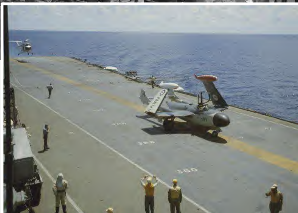
Shortly after landing, a Sea Venom taxis to its parking bay whilst simultaneously folding its wings. A Sycamore, probably the duty SAR helicopter, lands astern (Image: Kim Dunstan).→
