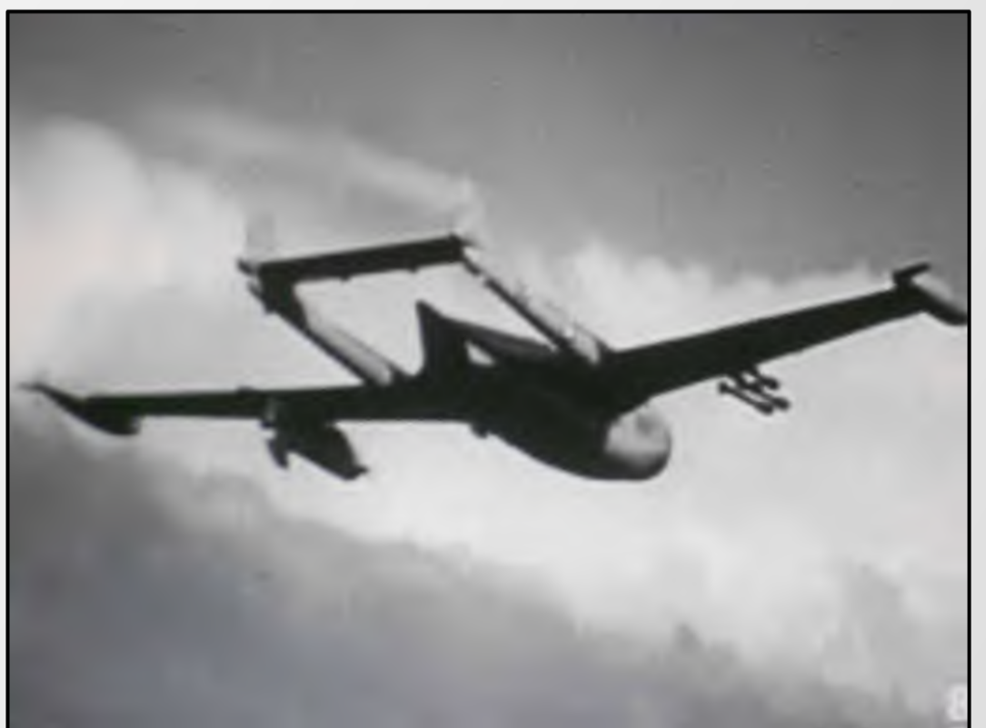
A Sea Venom during Ikara trials, conducted at Woomera and Port Wakefield from about February 1961. The weapon being tested is under the port wing, with 3 inch rockets under the starboard wing. (Phil Thompson collection). See a short video of the Ikara test here .➔
