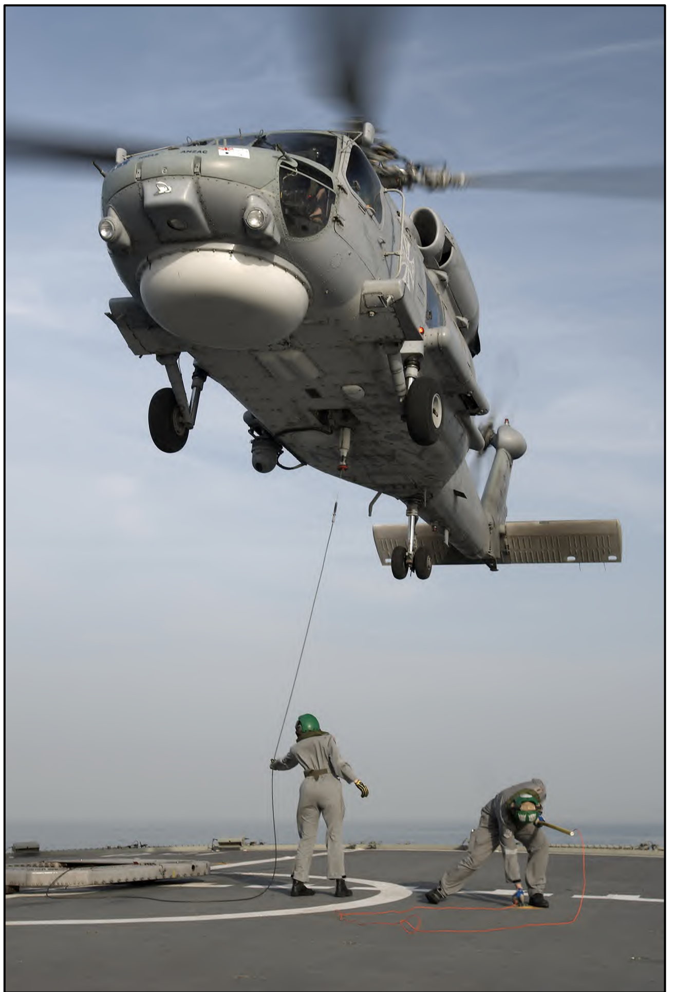
The Rapid Securing Device at work. The messenger cable has been lowered and attached to the RAST probe, which is being pulled into the aircraft - you can see it just under the fuselage. Once it has been secured the Haul Down cable, shown here being held by the figure in the green hat, will be tensioned and then, when the pilot is ready, the aircraft will be pulled onto the deck, aligning with the RAST trap on the LHS. →
