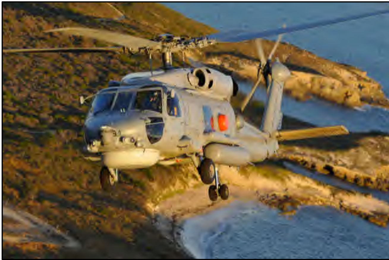
Left. An S-70B-2 off Garden Island, WA showing its Mid-Life Upgrades including FLIR, ESM/ECM and SAR Emergency Location Beacon. Below. A Seahawk over the deck of an RAN Anzac Class frigate, which could only carry one aircraft. Note the RAST shuttle immediately below the fuselage. →
