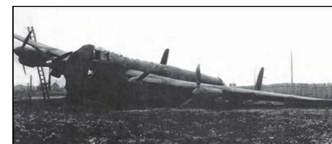
Middle. One of the Lancasters which landed at Belomorsk instead of Yagodnik. The undercarriage collapsed on the rough wooden planking of the airstrip, although the crew were uninjured.
