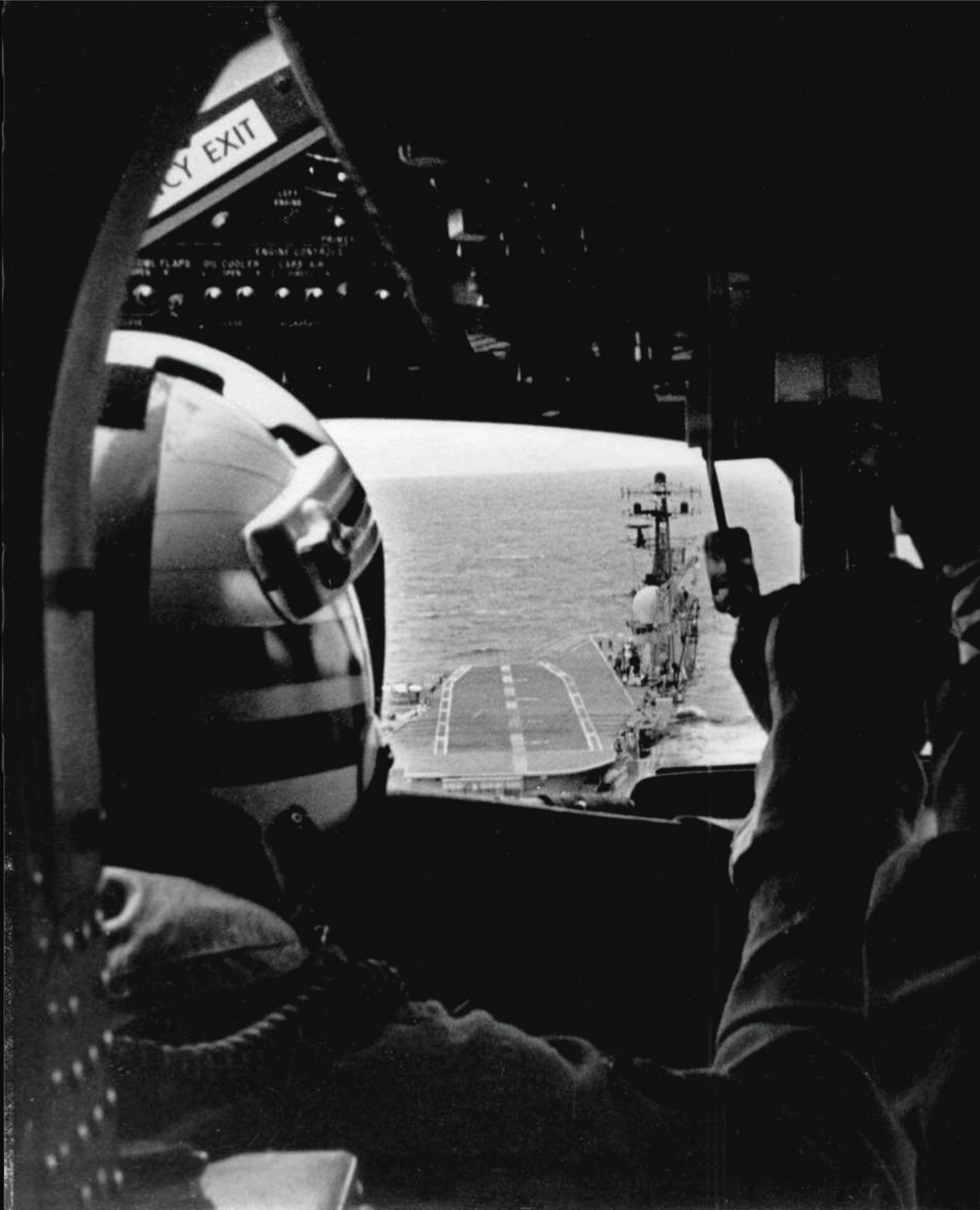
Above. Looking spick and span, HMAS Melbourne steams on a calm ocean whilst operating her new aircraft. A Tracker is about to capture an arrestor wire, whilst other Trackers and Skyhawks are secured in the parking areas forward and aft of the island. Once again, this photo illustrates how little room there was to operate modern aircraft aboard a light fleet carrier. (Photo: Fred Tyler). ➔
