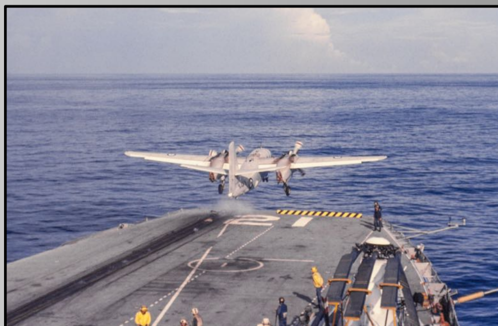
Above Left. This Tracker has been correctly marshalled onto Melbourne's single catapult and braced ready for take off. Above Right. Once pressure is released into the catapult piston the weak link in the holdback fitting breaks, and the aircraft is flung into the air (above right). →
