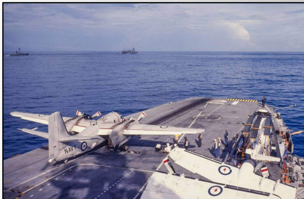
Above Left. This Tracker has been correctly marshalled onto Melbourne's single catapult and braced ready for take off. Above Right. Once pressure is released into the catapult piston the weak link in the holdback fitting breaks, and the aircraft is flung into the air (above right). →
