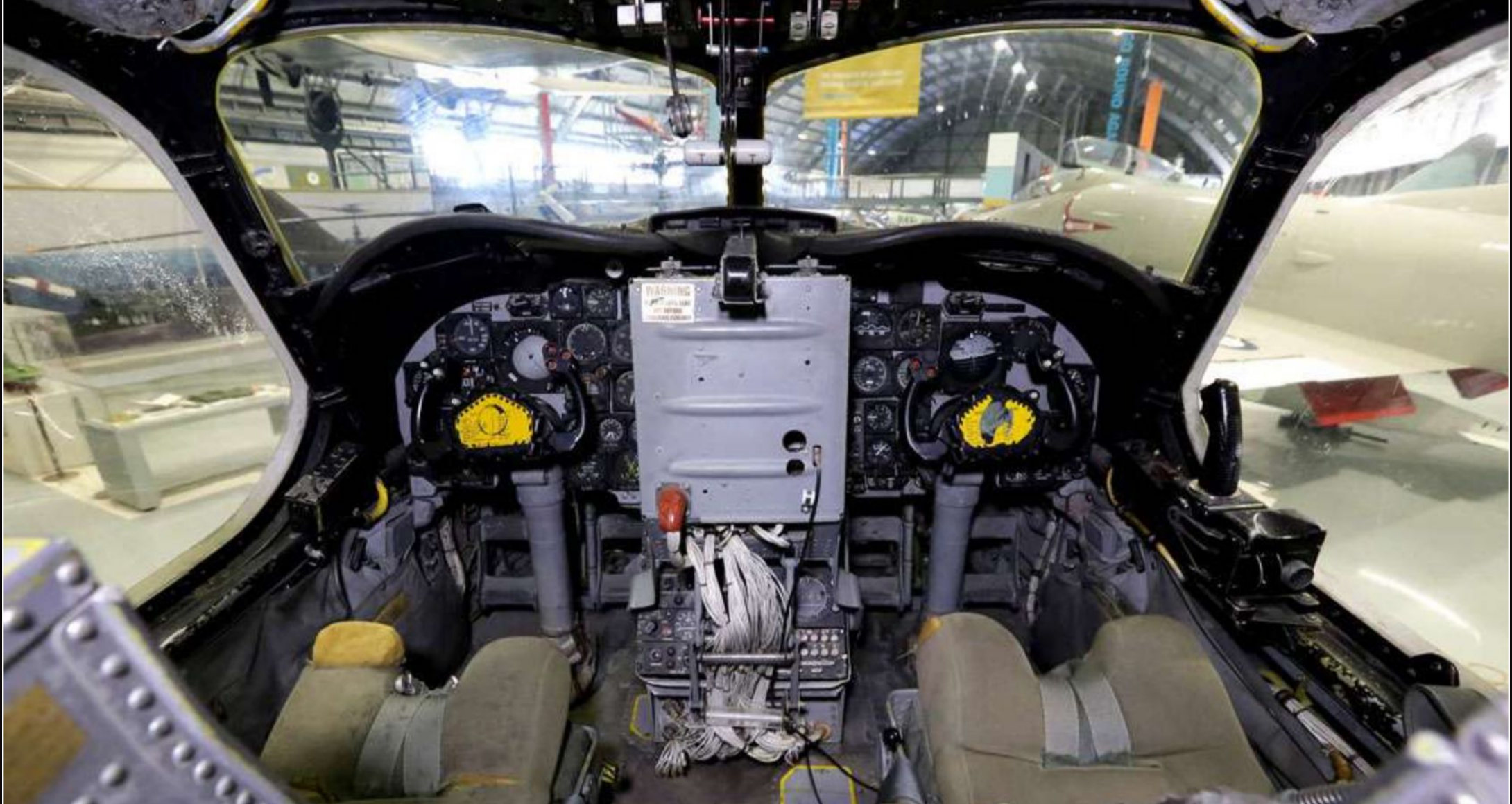
Above. A good shot of the cockpit of an S2E/G, lifted from an American ESO website page, somewhat ironically as it appears to have been taken in our own FAAM. The cockpit layout was conventional with the captain sitting in the left seat but the aircraft capable of being flown from either. Instruments were, of course, analogue. the fold up centre console can be seen in the 'up' position to aid access to the seats; when rotated downwards is provided mostly armament control functions – for example, sonobuoy release, torpedo depth selection and so on. We would welcome a more informed description of the image, should anyone wish to do so. Image courtesy of FLECOMPRON TWO. ➔
